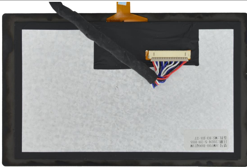
Figure 54 Connect LVDS screen cable to LVDS screen
