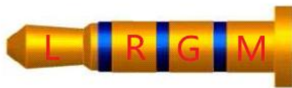
Figure 17 Definition of four-segment headphones
